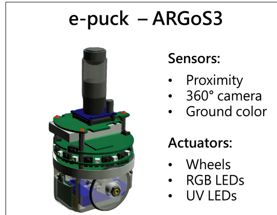
Figure 13: The e-puck robot considered in the experiments, along with its sensors and actuators. The picture shows the simulated version of the physical robot.
